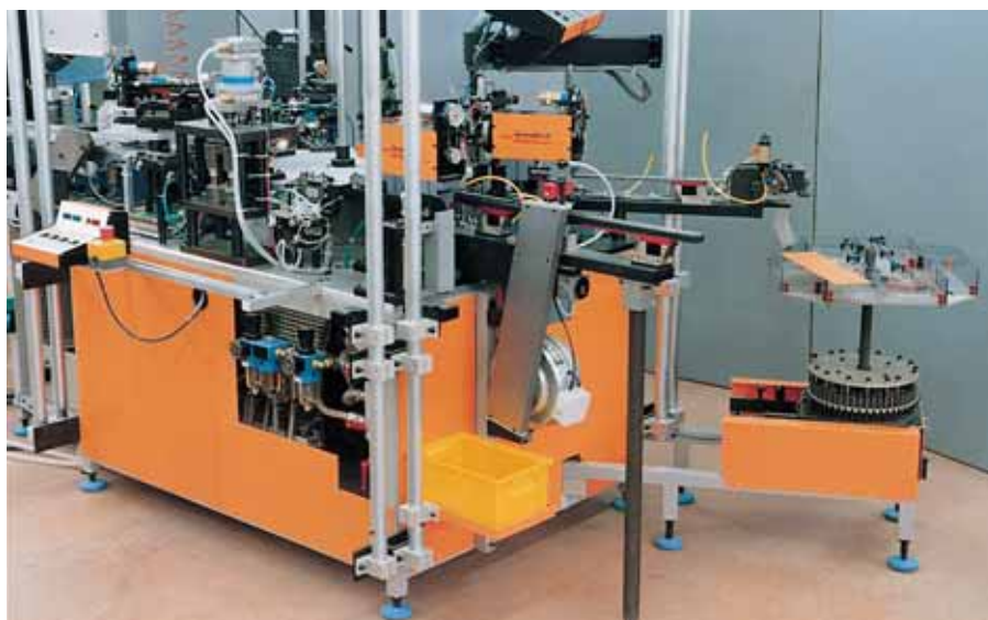
Protective covering guide device on automatic assembly unit, with weight compensation in the aluminium tubes.
