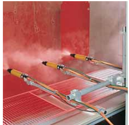
Spray fixture in a powder coating unit. The low weight of the fixture keeps the acceleration and deceleration forces down. The joints have good electrical conductivity properties.
