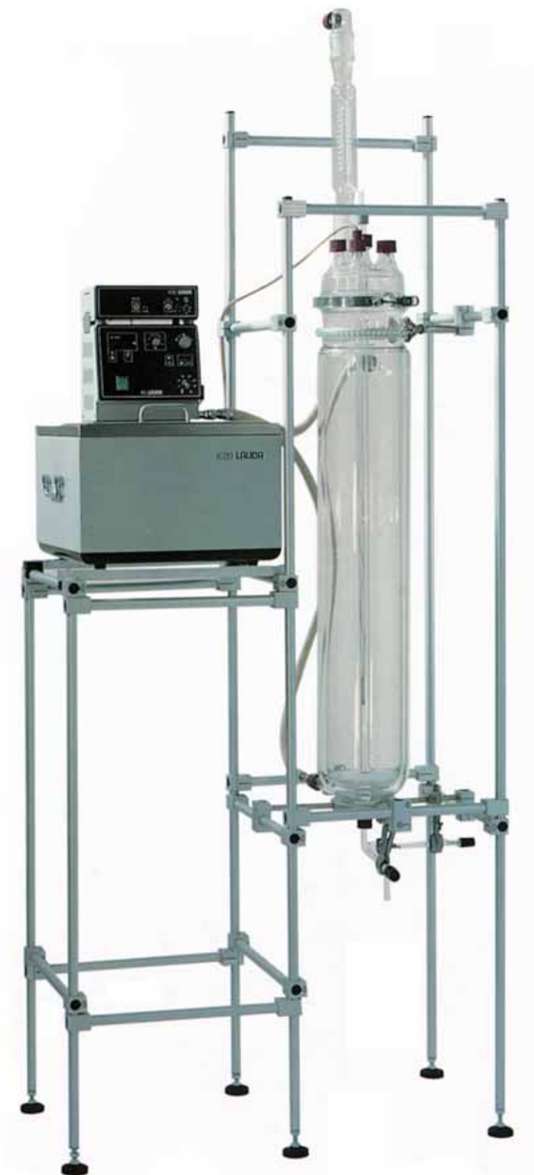
Bubble column reactor for liquid / gas phase reactions, with a tempering sheath and gas absorption device.
