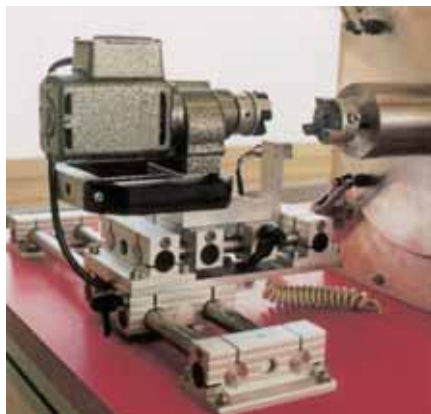
Couplable / decouplable drive on an X/Y adjustable unit for a micro-coating drum. The electric motor is in the decoupled position.
