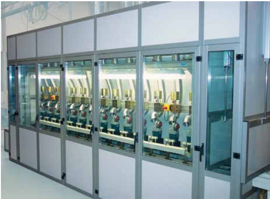
Endurance test bench for 2-hand angle grinder with noise protection screen locks
