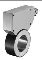
Thanks to its installation depth of only 20 mm, the bearingless magnetic rotary encoder RLA50, comprising a magnetic ring and sensor head, is ideally suited for plants and machinery where space is very tight. The non-contact measuring principle allows for error-free use even under harsh environmental conditions, as well as ensuring a long service life.
