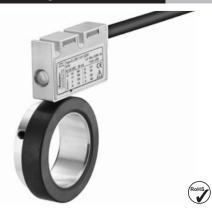
Thanks to its installation depth of only 16 mm, the bearingless magnetic rotary encoder RI50 / Limes LI50, comprising a magnetic ring and sensor head, is ideally suited for plants and machinery where space is very tight. The non-contact measuring principle allows for error-free use even under harsh environmental conditions, as well as ensuring a long service life. In contrast to our measuring system RI20 / Limes LI20, a single zero pulse is also implemented here.
