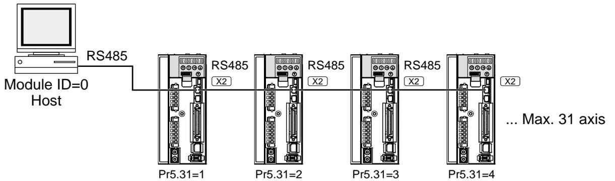
**Allow 50ms or longer interval for switching the axes while capturing data of multiple axes.**
