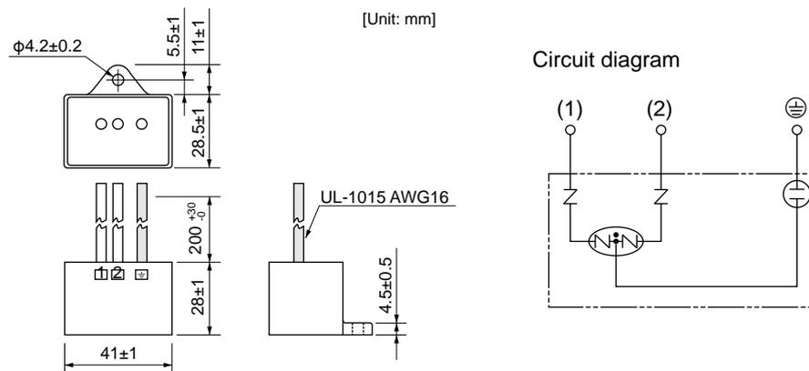
**Remarks** Take off the surge absorber when you execute a dielectric test to the machine or equipment, or it may damage the surge absorber.
