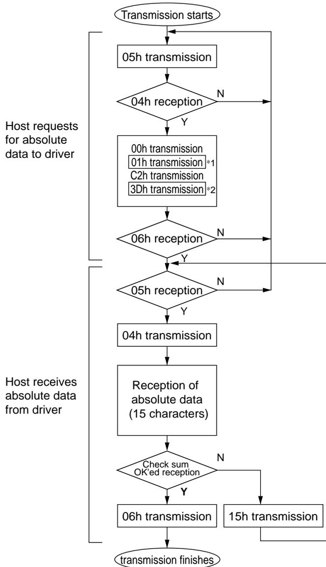
Data of \*1 and \*2 are determined by the setup of Pr5.31 "Axis address" of the front panel.
