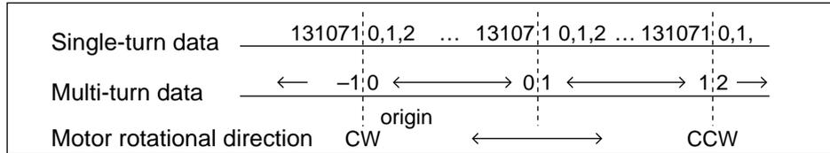
Single-turn data and multi-turn data are composed by using 15-character data (hexadecimal binary code) which are received via RS232 or RS485.
