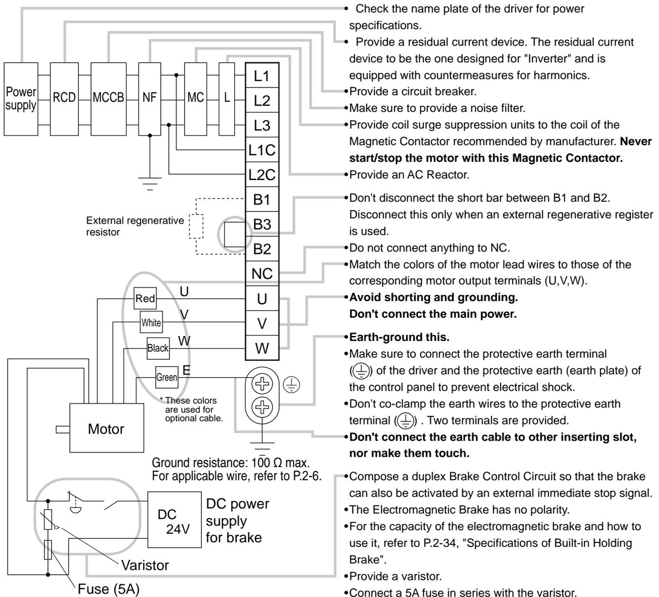
Compose the circuit so that the main circuit power will be shut off when an error occurs.
