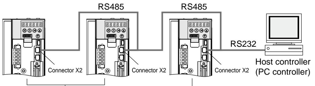
Set the axis number (Pr5.31) of driver to be connected through RS485 to a value in the range 1 to 31.
