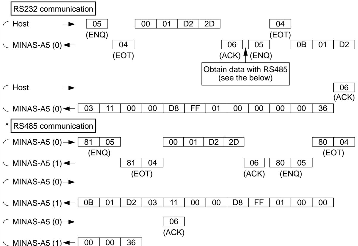
**Caution** See the below for the captured data. Refer to P.7-48, "Read out of Absolute Encoder" of details of communication command, for the data composition.
