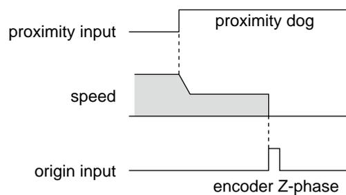
Proximity dog off... .Decelerates at an entry of the proximity input, and stops at an entry of the first origin input (Z-phase) after the input is turned off
