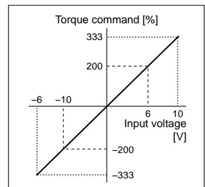
$$\text{Torque command (\%)} = 100 \times \text{input voltage (V)} / (\text{Pr6.00 setup value} \times 0.1)$$
