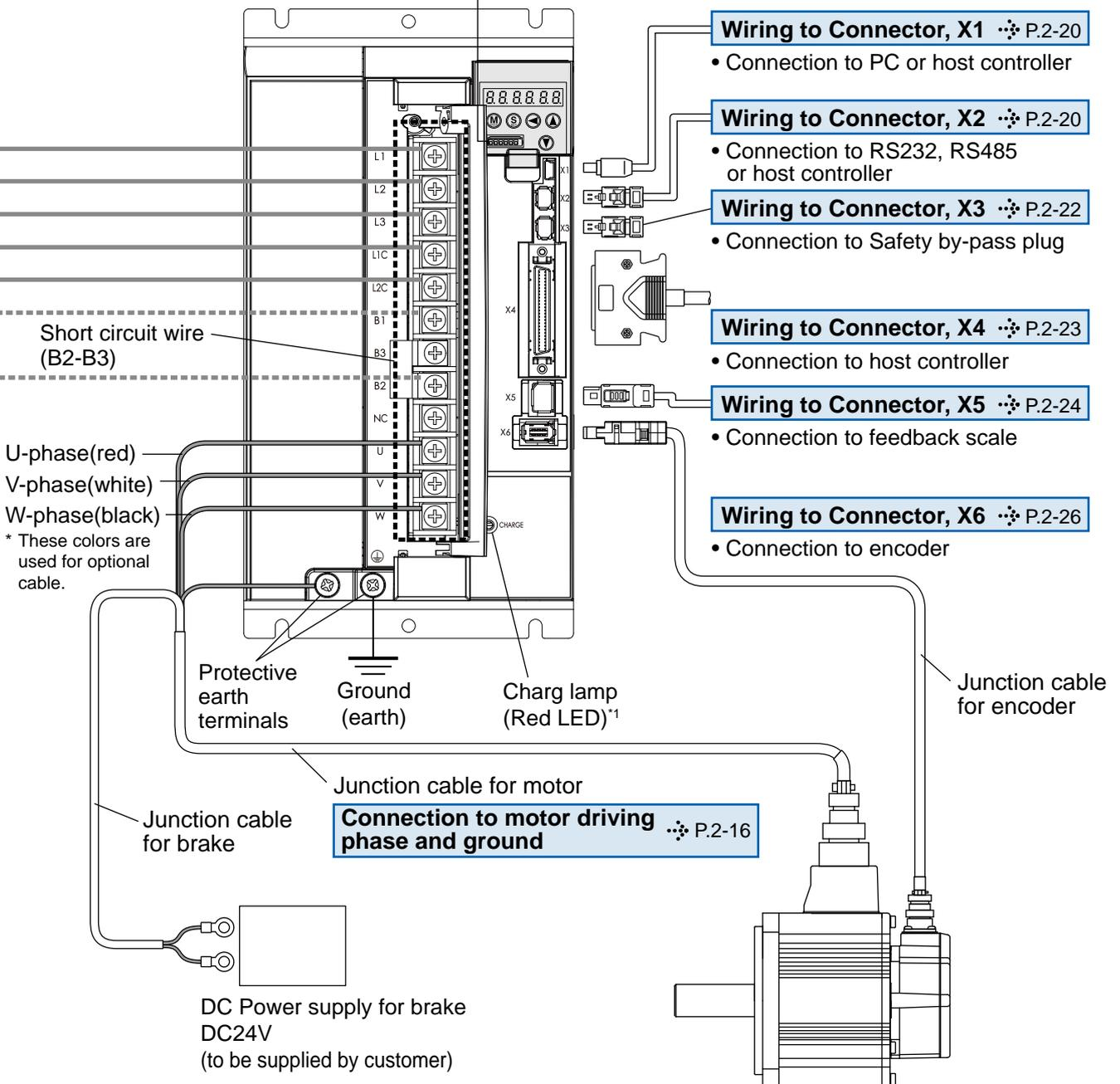
\*1 Do not make displacement, wiring or inspection while the LED is lit - cause of electric shock.
