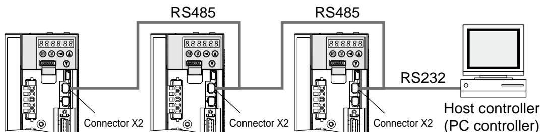
Set the axis number (Pr5.31) of driver to be connected through RS485 to a value in the range 1 to 31.
