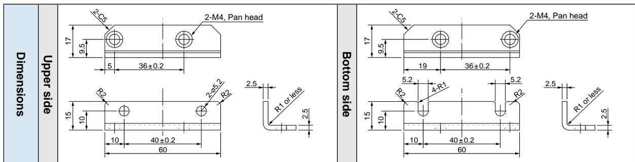
**Caution** For E and F-frame, you can make a front end and back end mounting by changing the mounting direction of L-shape bracket (attachment).
