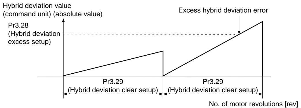
Note: Revolution in the hybrid deviation clear setup is counted by using encoder feedback pulses.
