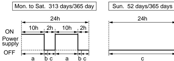
a : Current consumption in normal mode 3.6[ $\mu$ A]
