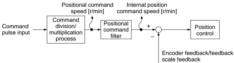
\*4 Command positional deviation is the deviation with respect to the command pulse input and the encoder positional deviation/ full-closed positional deviation is the deviation at the input section of the positional control, as described in the figure below.
