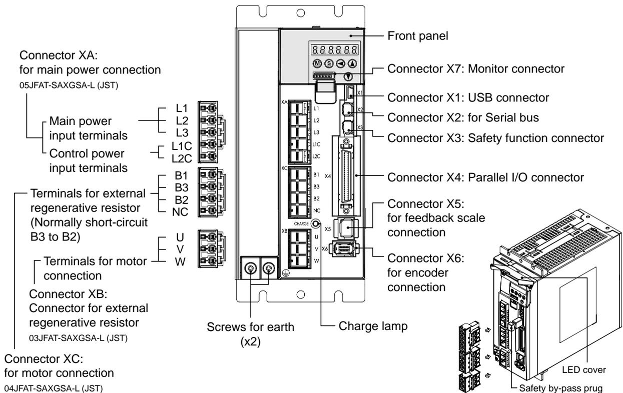
**Note** Connector X1 and X2 are attached in A to D-frame driver.
