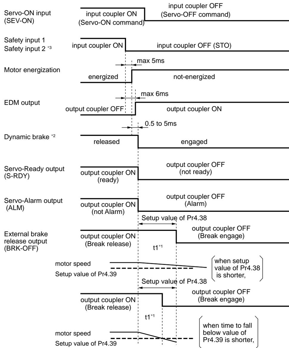
\*1  $t1$  is the value set to Pr4.38 Setup of mechanical brake action at running or the time at which the motor revolution speed drops below the time set to Pr4.39 Brake release speed setup, whichever comes first.
