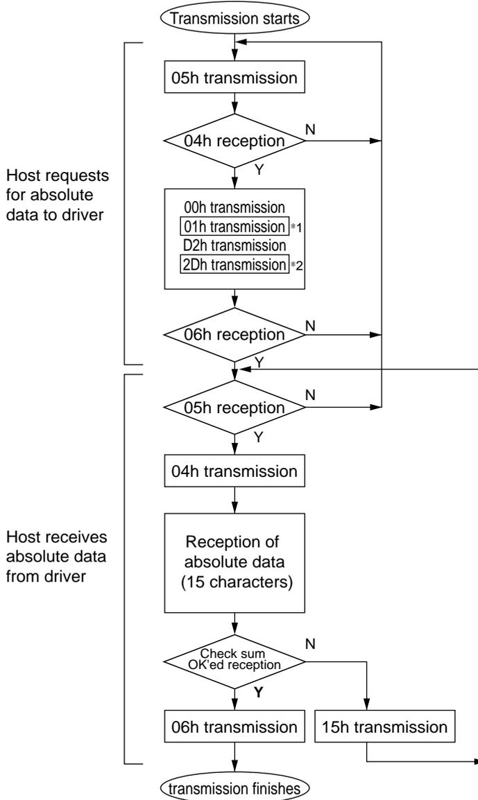
Data of \*1 and \*2 are determined by the setup of Pr5.31 "Axis address" of the front panel.
