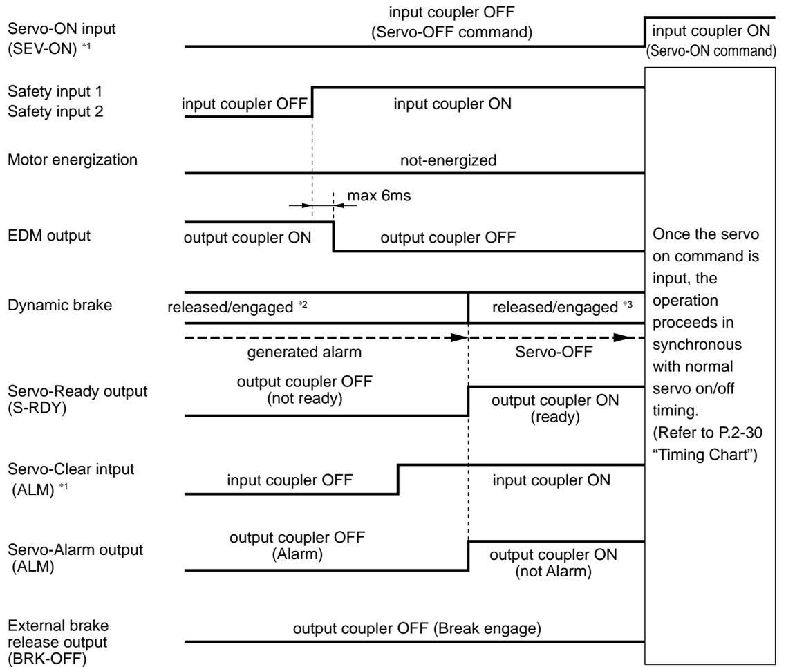
\*1 Photocouplers for safety input 1 and 2 should be turned on again with servo-on input turned off. Otherwise, alarm occurs, and should be cleared.
