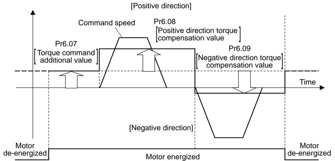
The friction compensation torque is the sum of the offset load compensation value which is set according to the torque command additional value (always constant) and the dynamic friction compensation torque which is set according to positive/negative direction torque compensation value.
