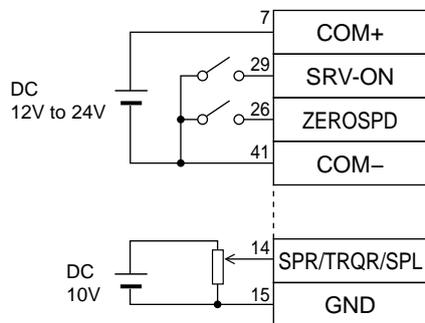
Run with ZEROSPD switch close, and Stop with open
