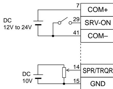
For bi-directional running (Positive/Negative), provide a bipolar power supply.
