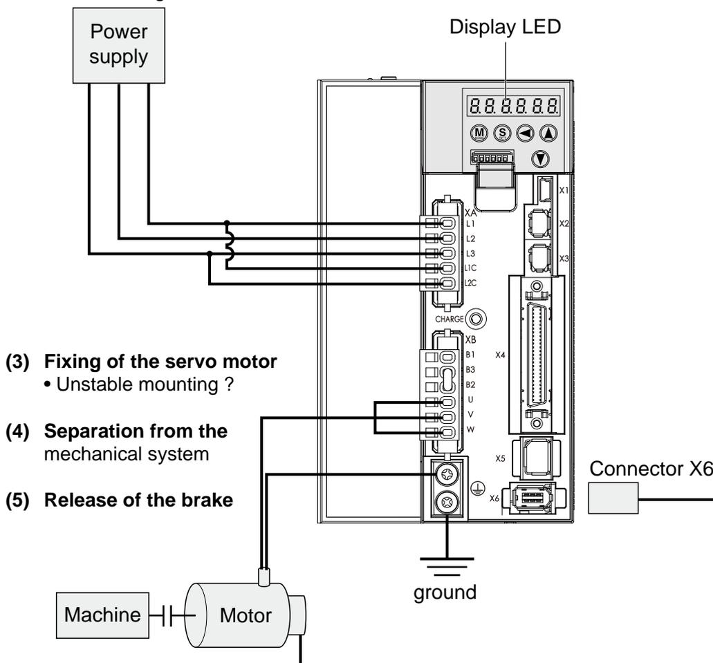
**(3) Fixing of the servo motor**
